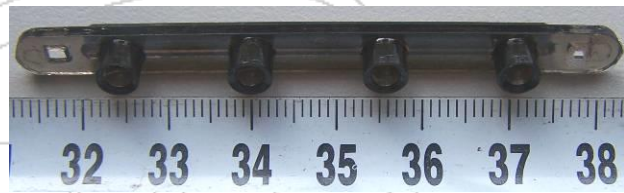
Photo 4: Indicator light board
